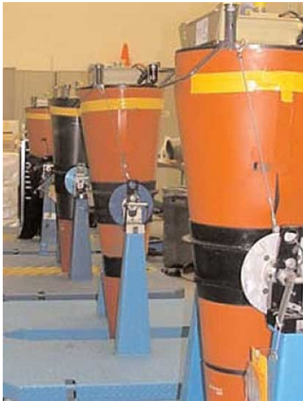
W76/Mk4a RBs on maintenance stands
